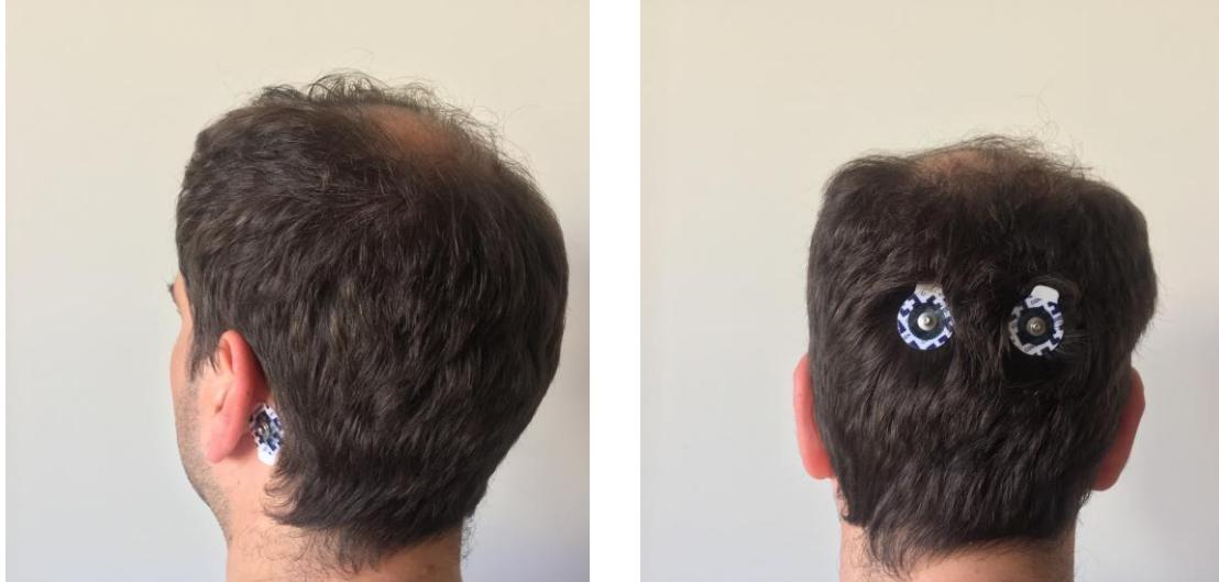
Fig. 4. Reference electrode placement on an electrically neutral location (left) and measurement electrodes (right) placed over the location of interest (the inter-electrode distance should not exceed 3 cm).
