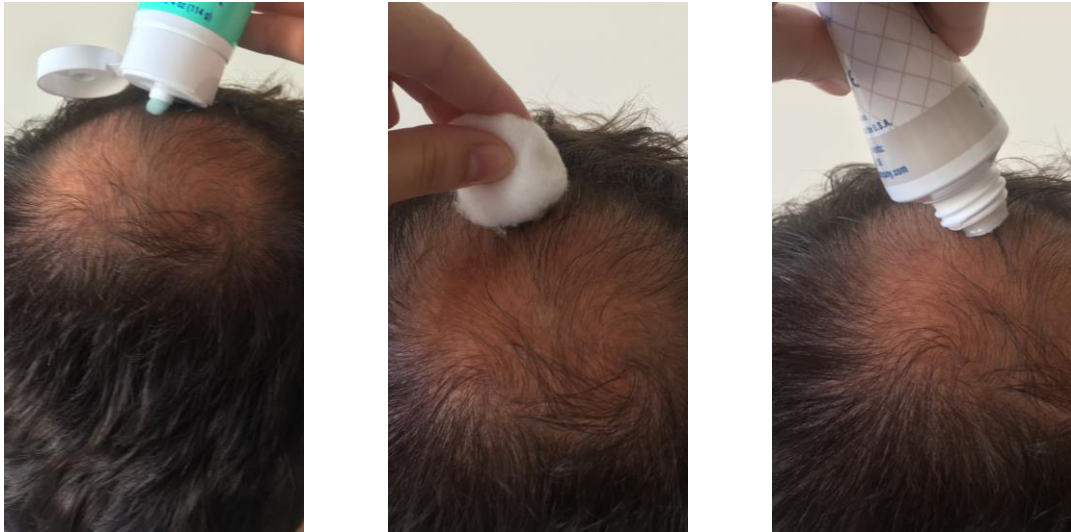
Fig. 6. Apply Nuprep skin preparation gel (left), exfoliate the scalp (center), and apply Ten20 conductive paste to improve the adhesiveness and conductivity... yes, bald spots are amazing for EEG ;)
