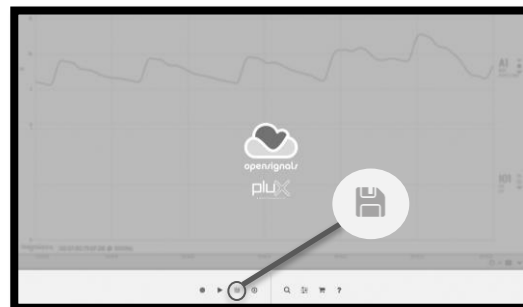
Fig. 5. Signal Storage Operation
