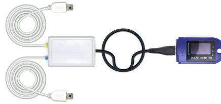
Fig. 1. User-friendly finger clip sensor for SpO2 and heart rate monitoring.
