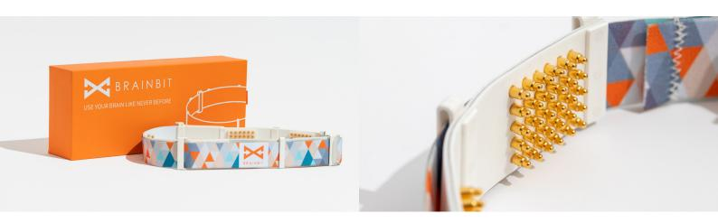
BrainBit Headband is a smart EEG device which monitors brain activity and gathers data that can be converted and used without professional help in reading. The headband has 4 dry EEG electrodes located at T3, T4, O1, O2 according to the international 10-20 electrodes placement scheme.
