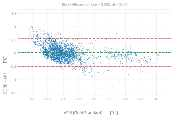
Figure 2: Bland-Altman plot showing the confidence interval for different core body temperature measurements of CORE compared to the ePill (Gold Standard)
