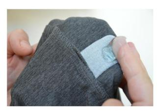
11. If you have a dry type of skin, to increase signal quality lubricate the textile electrodes on the inner surface of the Garment with a special gel.
