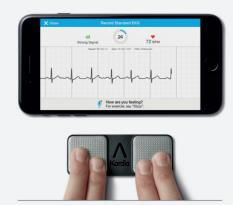
Place two fingers from each hand on each of the sensors to produce an ECG of lead I.
