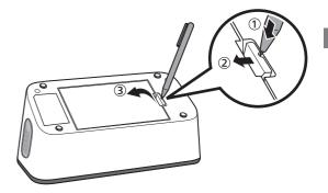
2. Insert 4 "AA" alkaline batteries as indicated in the battery compartment.
