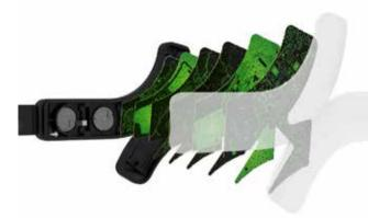
Six subsystem layers of QardioCore's next gen sensor system.
