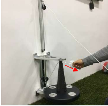
Put one end of the rope through the wall outlet block.
