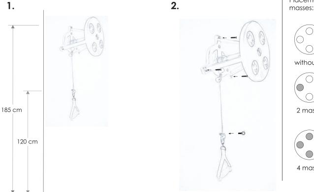
Place the top of the machine to an approximate height of 185 cm from de floor. Block wall outlet stands at 120 cm from the floor.
